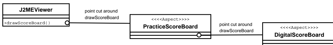
Figure 5.8: Practice Mode implemented using Aspects
