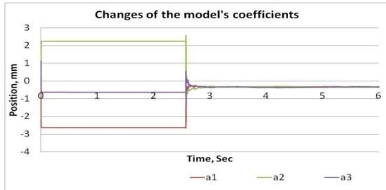
Fig 11: Changes of the denominator's coefficients of the model when noise was injected at 2.5 sec
