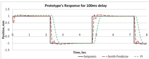
Fig 8: Prototype response using square wave reference
