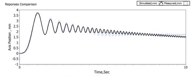
Fig 3: Measured (Dotted line) and simulated output (Solid line) waveforms
