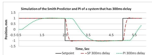
Fig 5: Simulation response with 300ms delay
