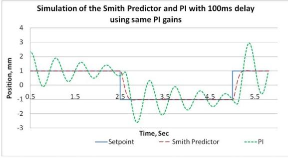
Fig 6: Simulation response with 100ms delay using same gains,  $P=16$  and  $I=0.5$
