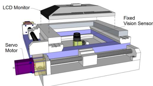
Fig 1: Vision sensor configuration
