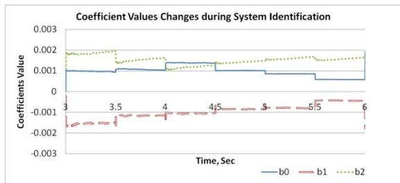
Fig 13 Changes of the numerator's coefficients of the model when noise was injected at 2.5 sec
