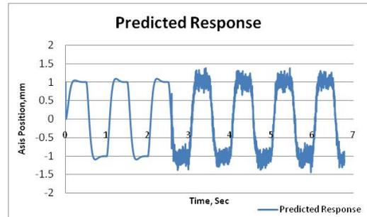
Fig 10: Online system identification model's output
