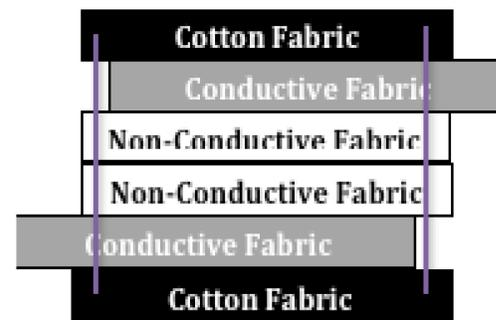
**Figure 4:** Pad design for current model.
