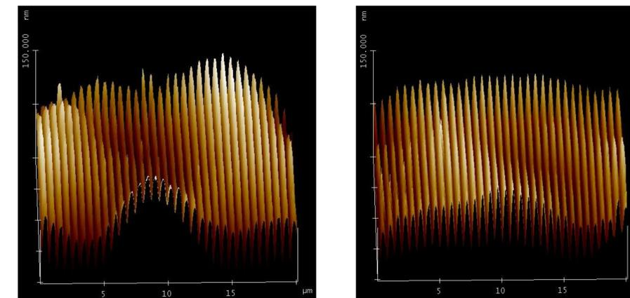
**Figure 4.** Effectiveness of creating a pattern on the membrane while deforming the membrane substrate. Common scale is 20 μm × 20 μm × 150 nm. The left image has an average channel height of 51 ± 19 nm, while the right image has an average channel height of 67 ± 11 nm.
