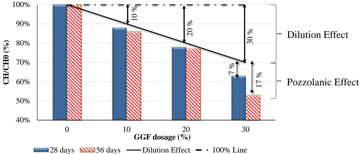
**FIGURE 2. Effect of GGF dosage on the TGA result [where CH is calcium hydroxide content of the sample and CH<sub>0</sub> is the calcium hydroxide content of the CTRL-1 (100% Cement)]**
