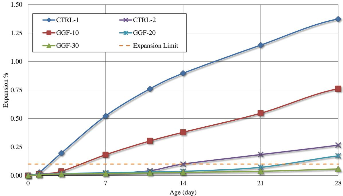
**FIGURE 3. Expansion of the mortar bar versus time**
