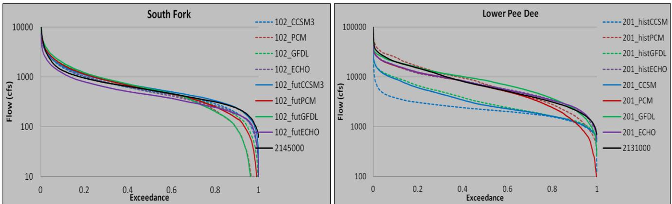
**Figure 1: Flow duration curves for South Fork and Lower Pee Dee rivers for the current (observed and simulated) and future intervals and observed gage.**
