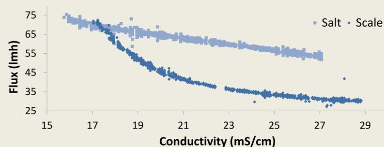
Figure 3: An example of a scaling experiment. NaCl does not produce scales and flux decline is linear with increasing concentration. In scaling solutions, flux decreases both due to increasing concentration and scale formation.
