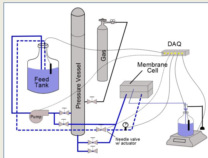
Figure 2: Sketch of bench-scale testing apparatus.
