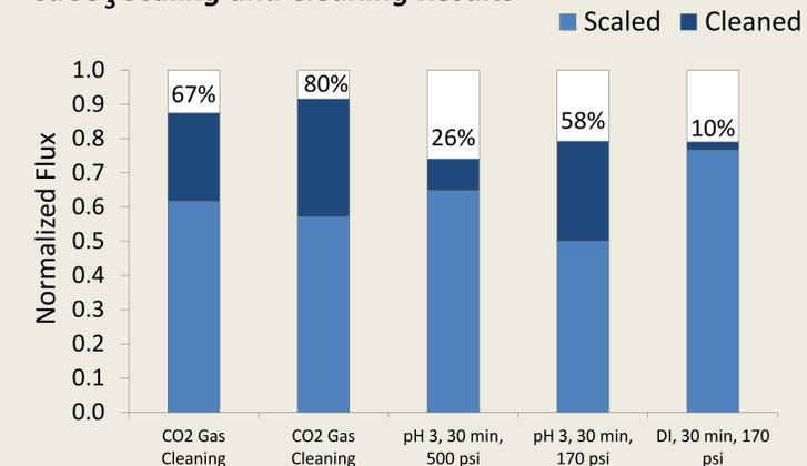
Figure 4: Comparison of cleaning efficiencies for membranes scaled by CaCO<sub>3</sub>. Cleaning with dissolved CO<sub>2</sub> returned the most flux, followed by acid cleaning.
