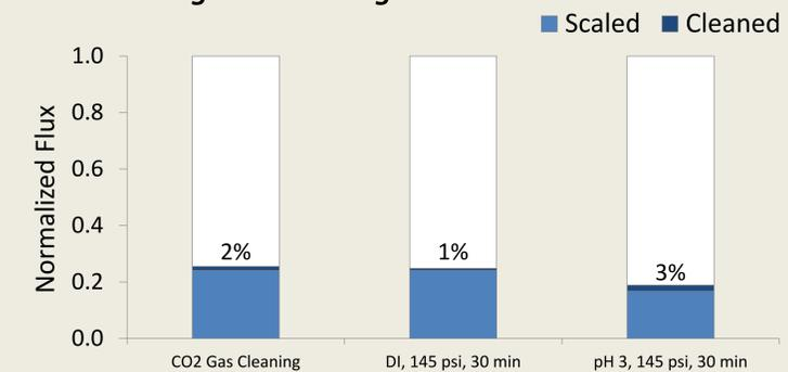
Figure 5: Comparison of cleaning efficiencies for membranes scaled by silicates. None of the attempted cleaning procedures regenerated flux.
