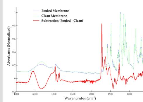
Attenuated total reflectance, Fourier transform infrared spectrometry (ATR-FTIR) is used to study organic functional groups on the membrane. Here, the clean membrane spectrum has been subtracted from the fouled membrane spectrum to reveal a sharp peak at about 1750 wavenumbers. The meaning of this and other peaks is still being investigated.
