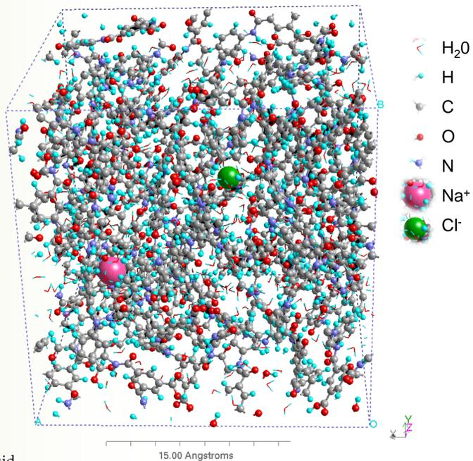
A molecular model (above) of the polyamide membrane active layer represents the surface to which foulants adhere. While the membrane chemical makeup is well characterized, the foulants are not. This project seeks to determine the foulant character and understand how molecular-level interactions affect the full-scale engineered system. (Image created by Andrey G. Kalinichev, University of Illinois at Urbana-Champaign. Used with permission.)
