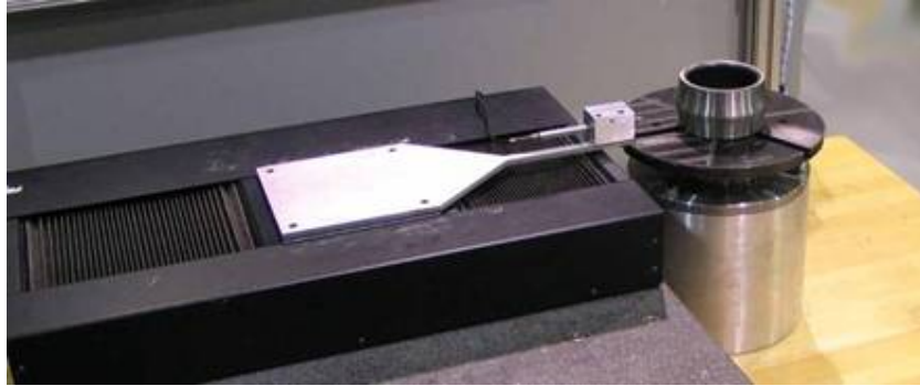
Figure 1 - Prototype System: Spindle, Linear Slide, Measurement Probe, Pusher Tip
