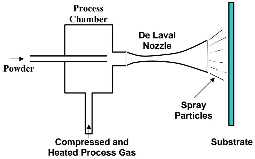
**Figure 2. A schematic of the Cold-gas Dynamic-spray process.**
