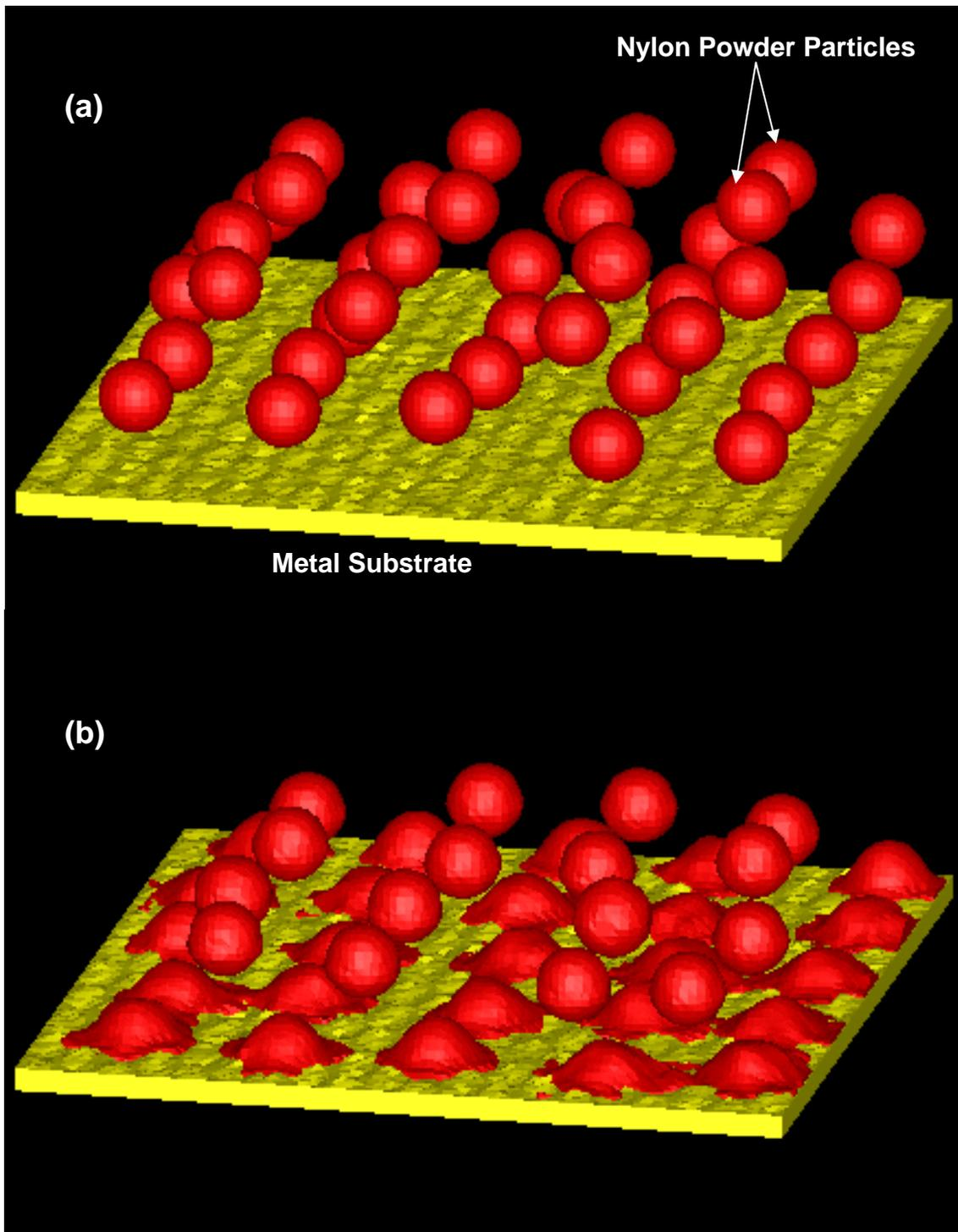
**Figure 6. Temporal evolution of the coating and substrate materials during cold-gas dynamic-spray: (a) 0ms; (b) 0.1ms; (c) 0.2ms; and (d) 0.3ms.**
