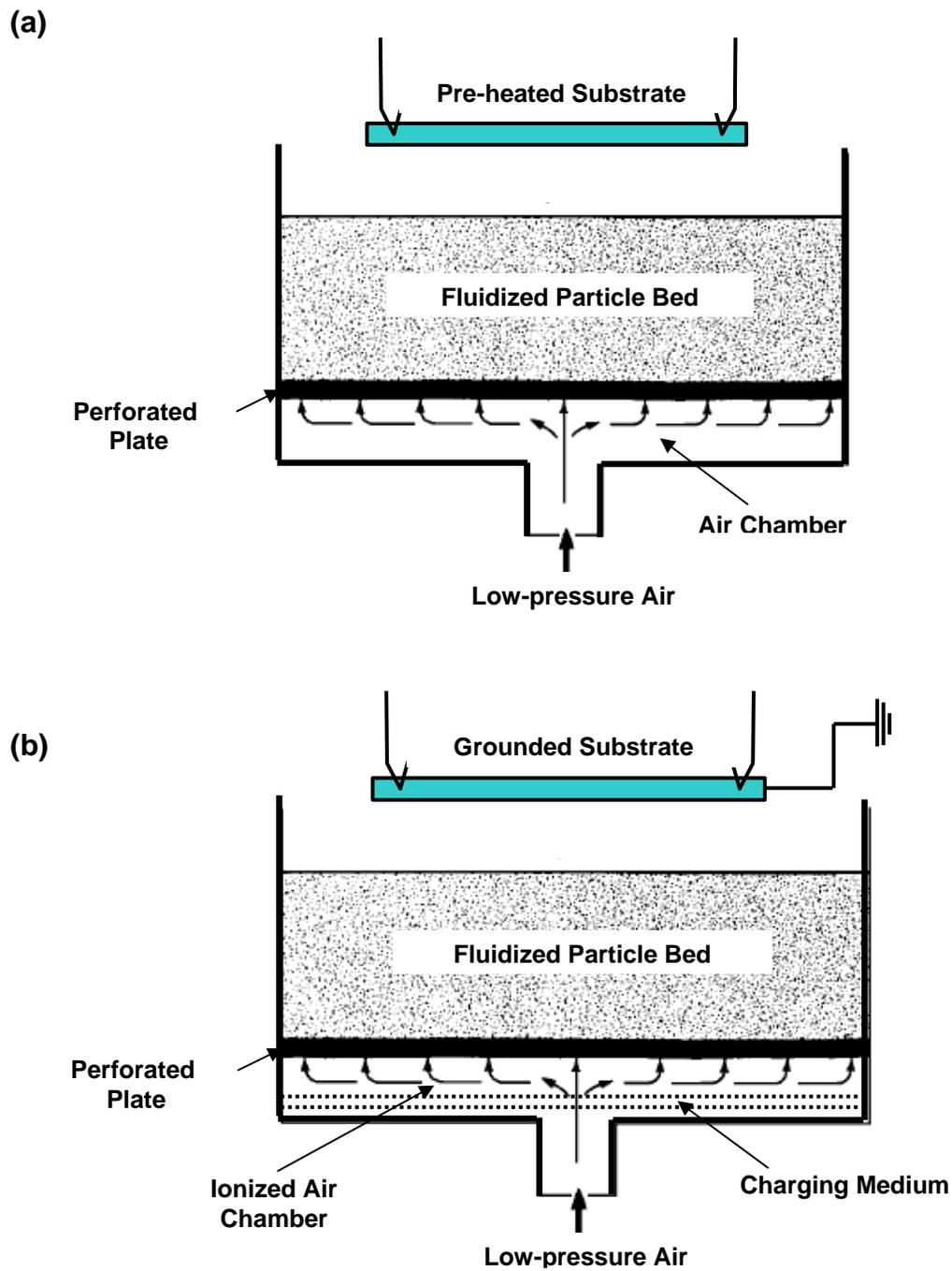
Figure 4. A schematic of the: (a) Conventional and (b) Electrostatic Fluidized-bed process.
