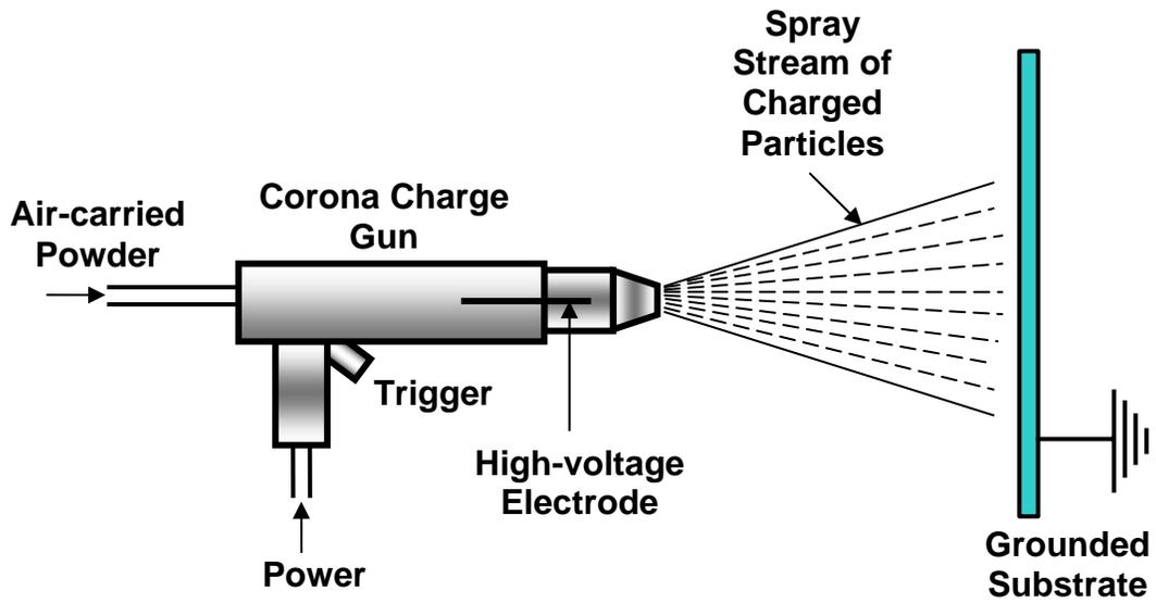
**Figure 3.** A schematic of the Corona Spray process.
