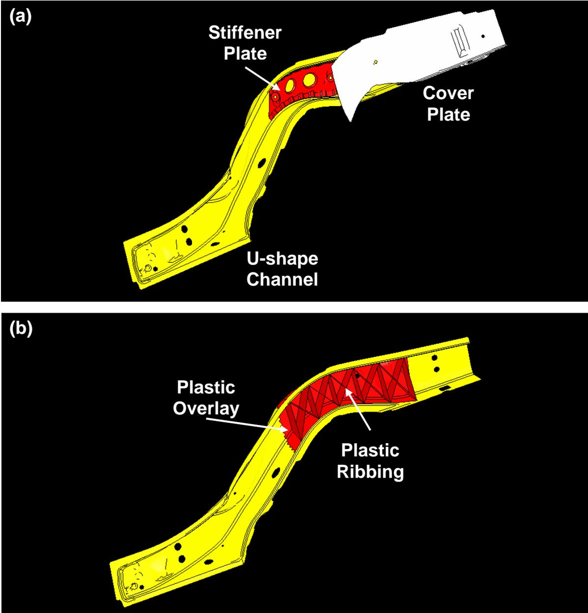
Figure 1. An example of the: (a) All-metal and (b) PMH load-bearing automotive component.
