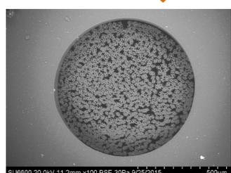
Cross-section of C-CP fibers under SEM
