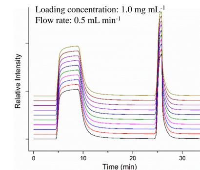
Figure 4. Column to column consistency
