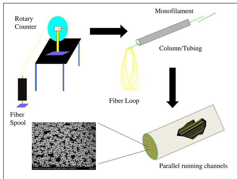
Figure 1. C-CP fiber column construction process
