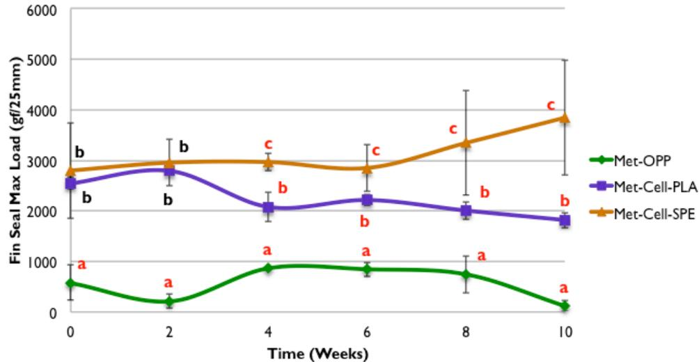
**Figure 13:** Fin seal strength max loads (gf/25mm) of three different packaging materials stored over time
