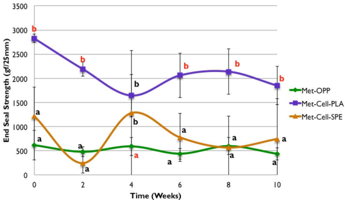
**Figure 12:** End seal strength max loads (gf/25mm) of three different packaging materials stored over time (Within the weeks, the packaging materials with the same letter are not significantly different.)
