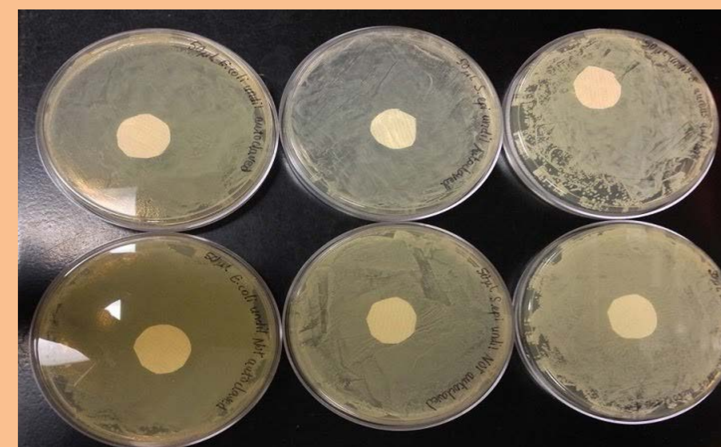
Figure 1. Test to determine if the Tyvek lab coats contained antimicrobial properties that would inhibit bacterial growth using pieces of lab coats both autoclaved and not. This figure suggests the Tyvek lab coats do not have antimicrobial properties
