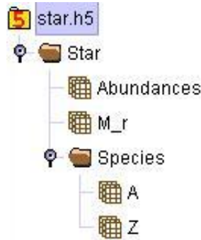
Figure 4.1 This Figure is a screenshot of the input HDF5 file for the wn_1d_stellar_ejecta module as seen in HDFview. The file contains all of the abundances of the star’s species as a function M_r .
