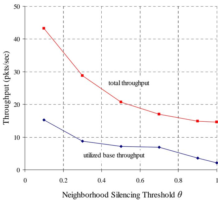
(b) Throughput vs.  $\theta$ Figure 4.21 Performance of 4000 by 4000 network with  $Q = 20$  and  $\alpha = 3$
