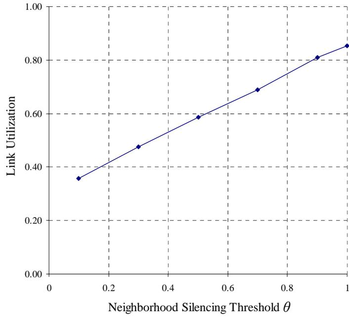
(a) Link utilization vs.  $\theta$
