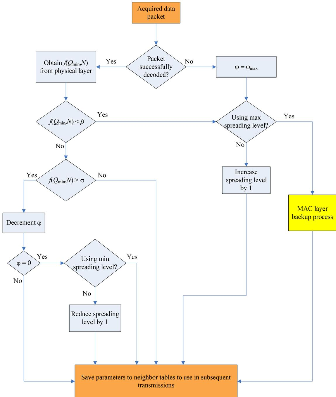
Figure 2.1 Adaptive-transmission protocol operation when multiple-access interference is detected
