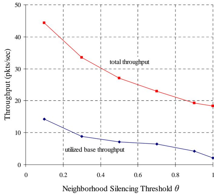
(b) Throughput vs.  $\theta$ Figure 4.22 Performance of 6000 by 6000 network with  $Q = 20$  and  $\alpha = 3$
