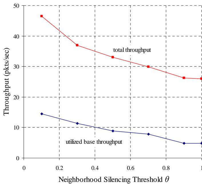
(b) Throughput vs.  $\theta$ Figure 4.23 Performance of 8000 by 8000 network with  $Q = 20$  and  $\alpha = 3$
