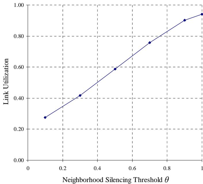
(a) Link utilization vs.  $\theta$
