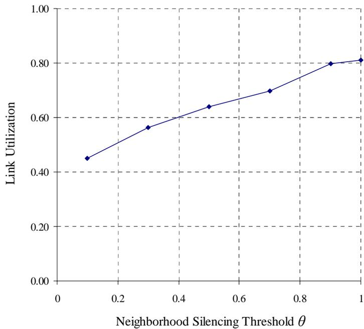
(a) Link utilization vs.  $\theta$
