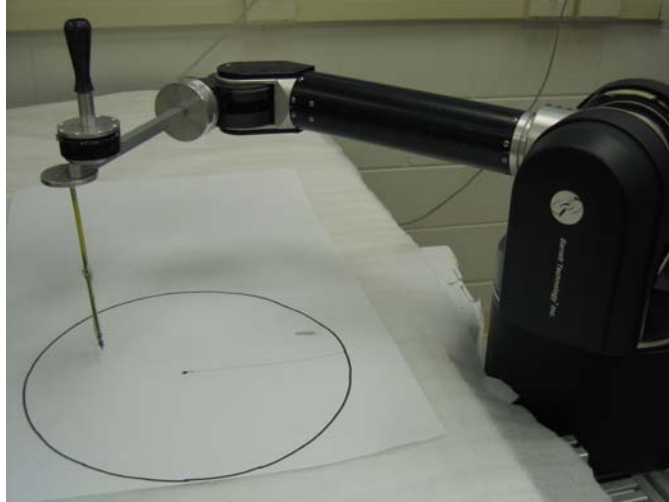
Figure 4.1: Barrett whole arm manipulator
